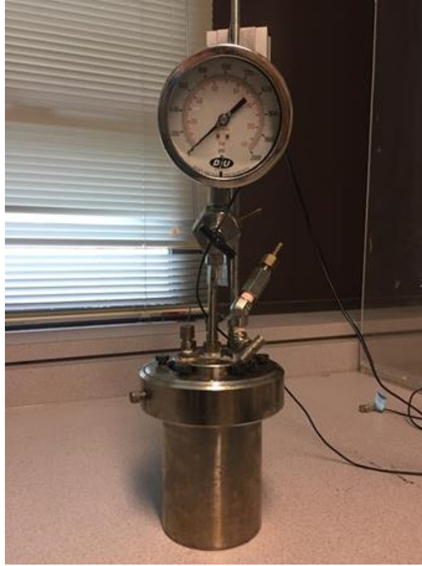
Figure 3-9: Electrochemistry autoclave used for experiments above 100 °C
